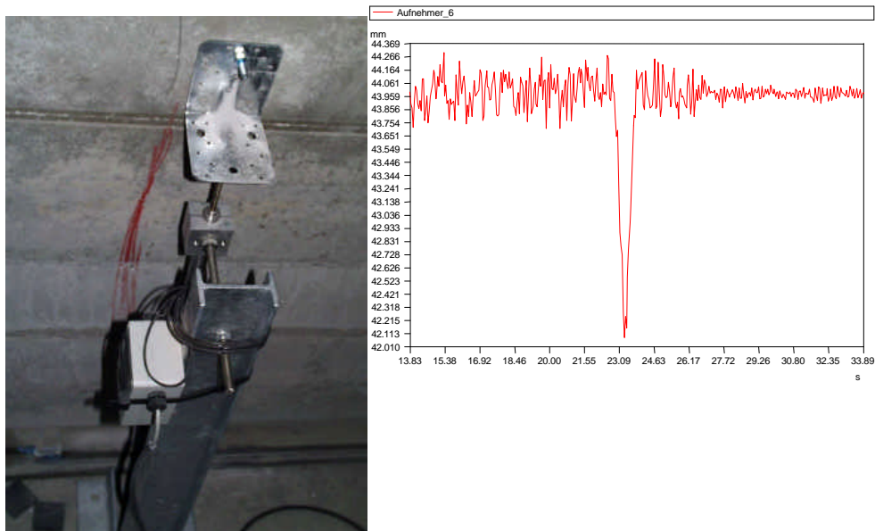
Figure 5. Sensors installed to the MSS – Results of measurement
