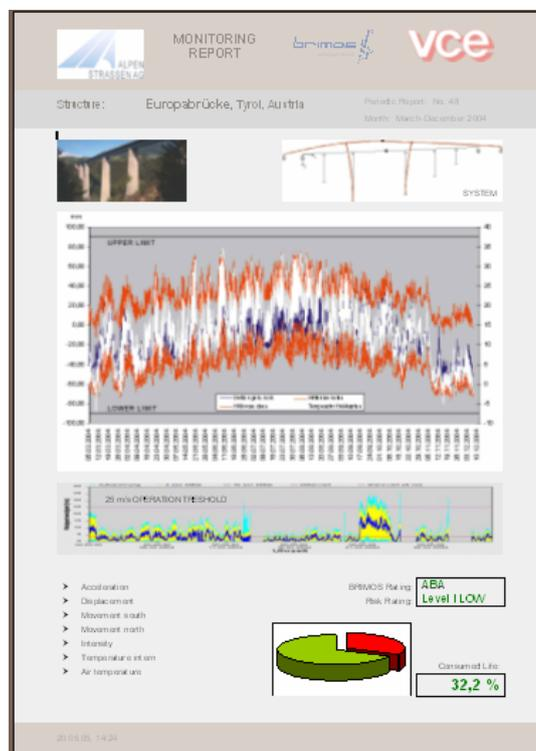
Figure 3: Typical periodic report for a bridge structure
